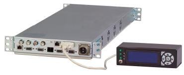
Front panel mounted in a small box (6" wide x 3" deep x 2" high) connected to main encoder body (8.625" wide x 28" deep x 1RU high) by a 25-foot remote control tether.
