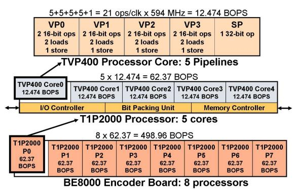
This includes the most compute-intensive motion estimation and motion compensation tasks performed on the multiple, adaptive macroblock sizes allowed by AVC coding. The 4x4 block intra-prediction algorithm, for example, calculates eight modes simultaneously, using the two arithmetical operations supported by each of the 4 vector pipes in a core—fully 8X faster than this particular algorithm could run on a single scalar unit.
